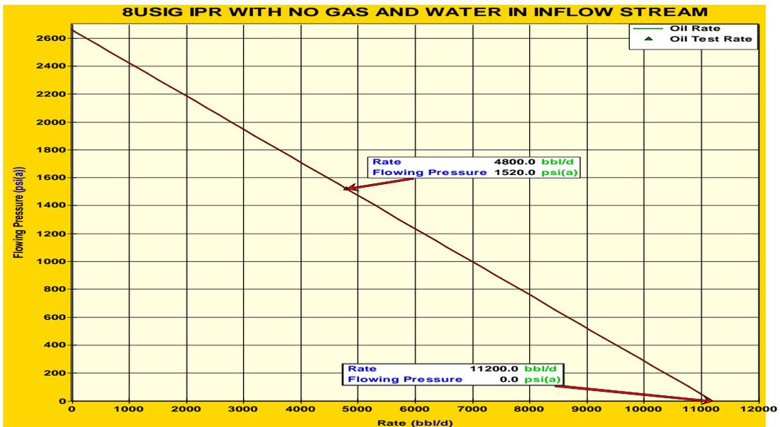
Fig.3: 8USIG IPR Curve for Single Phase Oil in the Inflow Stream.
