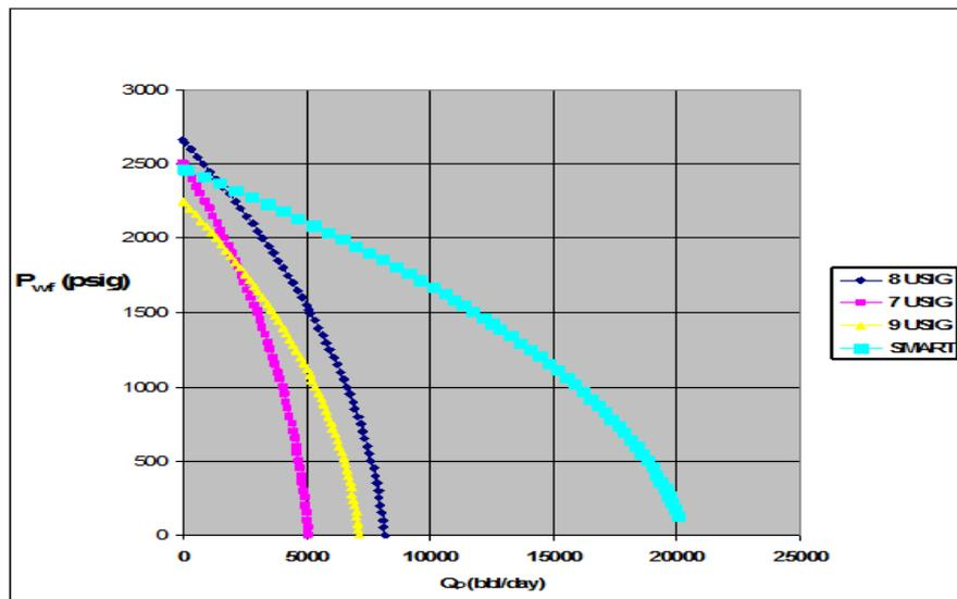
Fig.6: Producing Zones and Smart Well IPR Comparison
