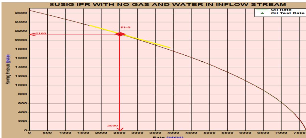
Fig.3: 8USIG PI Determination Curve
