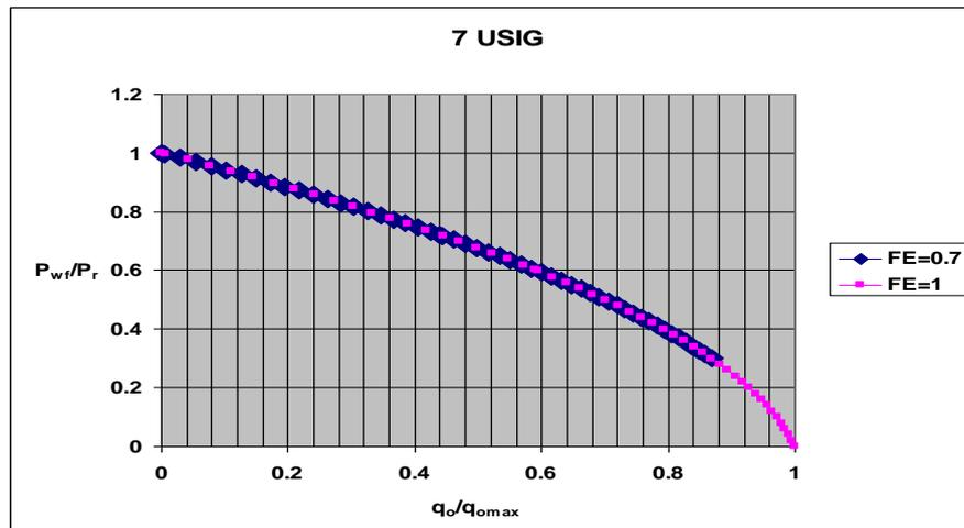
Fig. 5: 7USIG IPR in Terms of Changes in Flow Efficiency.
